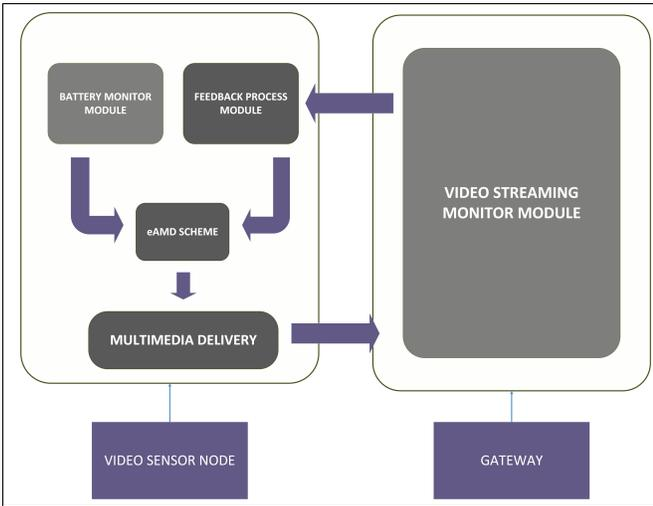
Fig. 2. eAMD-based system block-level diagram
