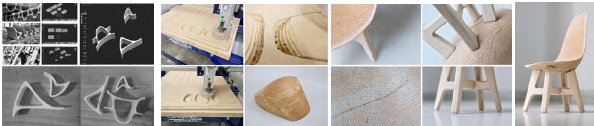
Figure 11. Design and fabrication of molds for making a structural beam (left) by Covadonga Lorenzo and fabrication of a chair (right) by Javier Buron. Photo credits licensed by Javi Buron García under a CC BY-NC-ND license.
