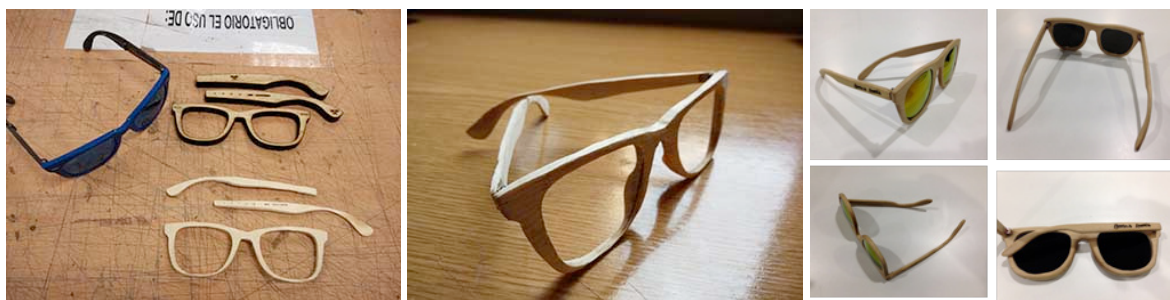
Figure 1. Design and fabrication of laser cut wooden glasses by Adolfo Gutiérrez (left and center) and Eduardo Chamorro (right). Photo credits: Adolfo Gutiérrez © 2014
