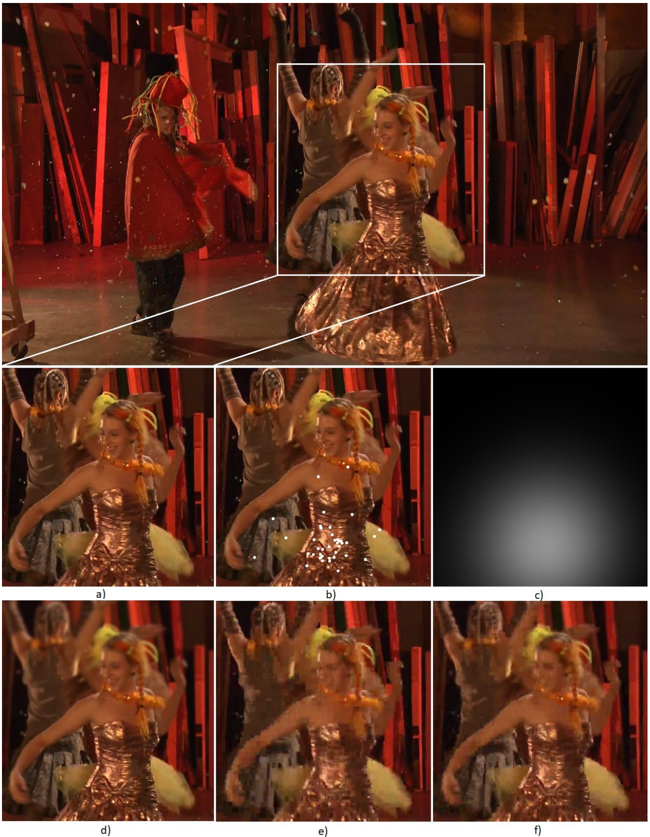
Figure 2. Frame examples demonstrating the encoding process of proposed method: a) original video frame, b) original video frame with white dots signalling eye tracker positions, c) saliency map created from eye tracker coordinates, d) blurring using saliency map, e) original video encoded with x264 codec with 1.5 Mbps, f) blurred video ( \sigma_n = 0.15 ) encoded with x264 codec with 1.5 Mbps.
