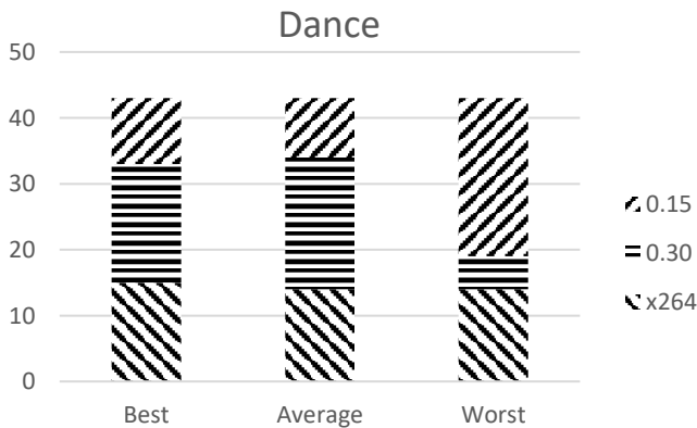
Figure 4. Quality of experience while watching Dance video with different blurring compared to regular x264 encoding.
