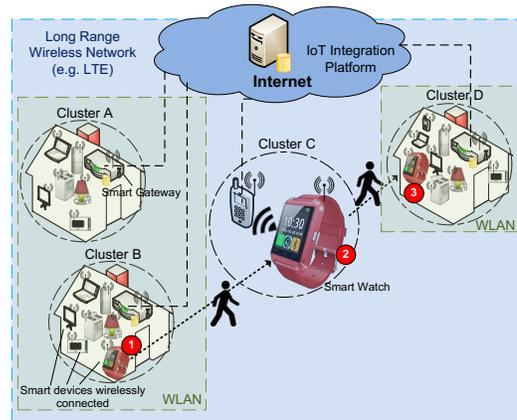
Fig. 1. ITMEMS's High Level IoT-based Architecture
